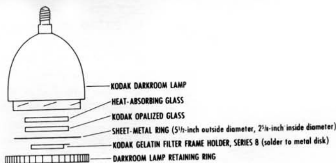
With a lamp, such as a Photo Enlarger Lamp No. 211, a modified KODAK Darkroom Lamp becomes a suitable light source for preflashing strips of film.
